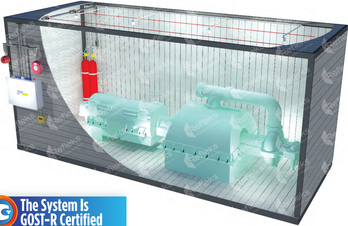
Container CO 2 Gas Extinguishing Application
